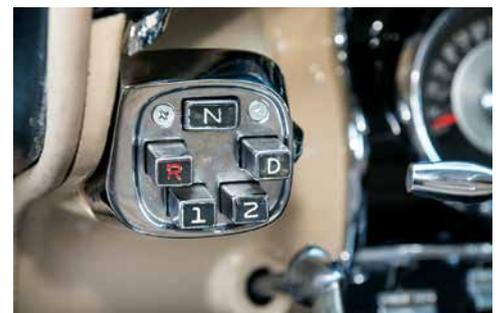
Pushing buttons to shift gears was a radical concept. At night, the button in use was dimmed, while the others around it were brightened.
